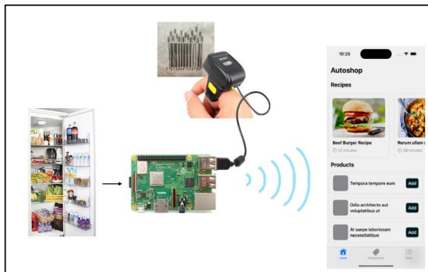
Figure 1. Working principle of the developed smart refrigerator
