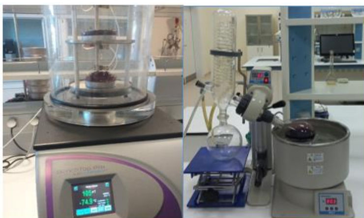
Figure 2. Freeze drying and vacuum rotary evaporation of berberis extract
